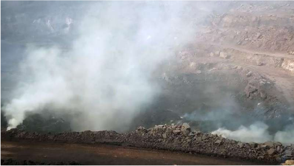
Figure 17: Coalfries in active seams in Kusunda (point 23 in figure 13 and table 4)
